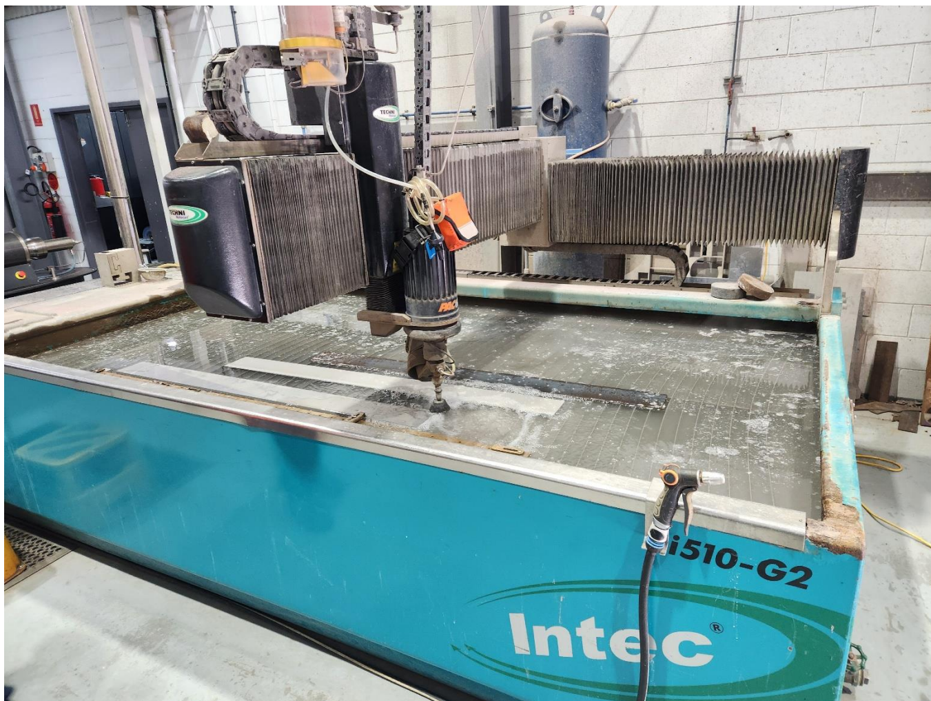
Figure 5: CSIRO Queensland (Engineering Workshop) Technijet - Intec 510-G2 waterjet cutting machine
