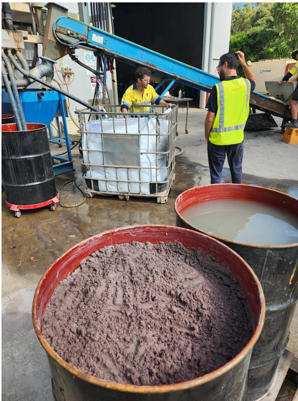
Figure 4: IHC processing Kanmantoo Mine bulk tailings Sample with Garnet Concentrate visible in drum
