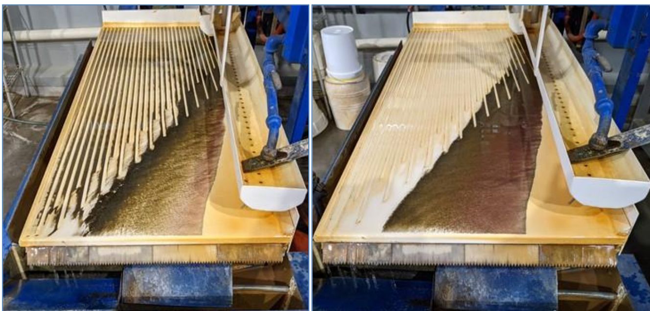
Figure 3: Image showing rougher (L) and cleaner stage (R) Shaking tables
