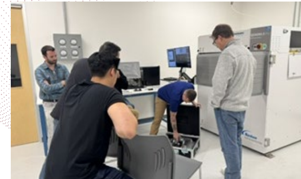
New x-ray machine for inspecting sealed assemblies
