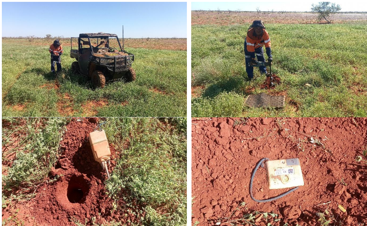
Images: Passive seismic nodes being positioned for data collection as part of 2026 Passive Seismic Survey
