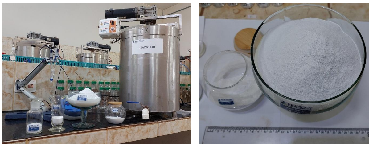
Figure 2. MREC precipitation cell (left) and final MREC product (right) produced at the BCM laboratories Brazil.
