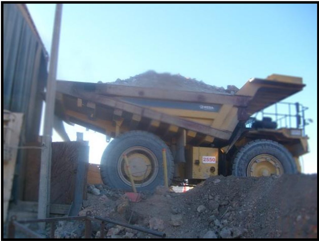
Figure 7 – Teck copper ore being dumped in the primary crusher
